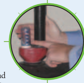
oil tank gauge
